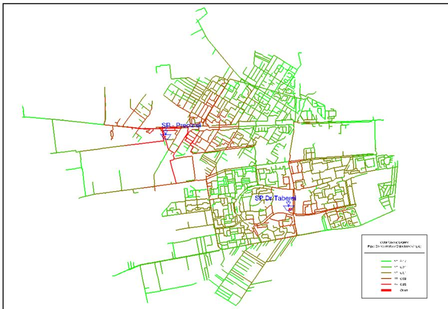
**Figure 2. Residual chlorine concentration in the water network model**
