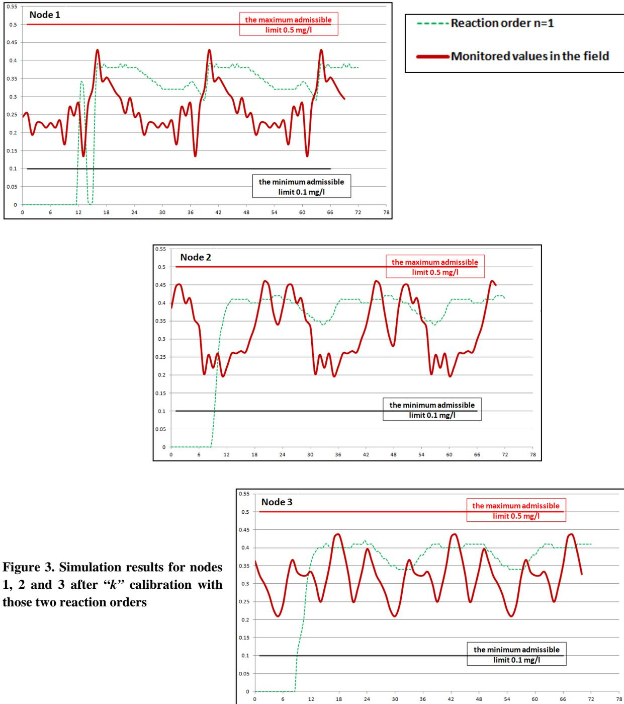
Figure 3. Simulation results for nodes 1, 2 and 3 after “ $k$ ” calibration with those two reaction orders
