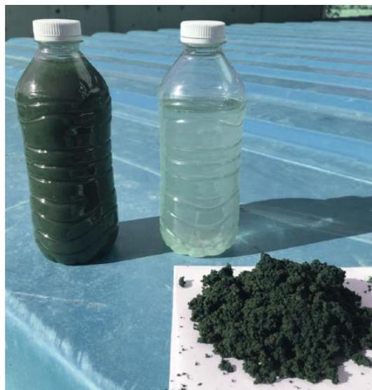
Figure 2. Left: Sludge before dewatering;
