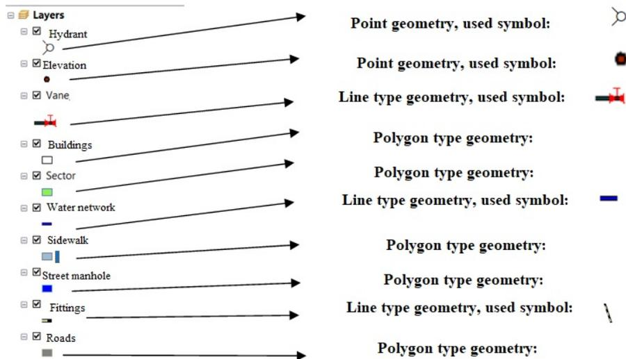
**Figure 2. Characteristic layers of the GIS model**
