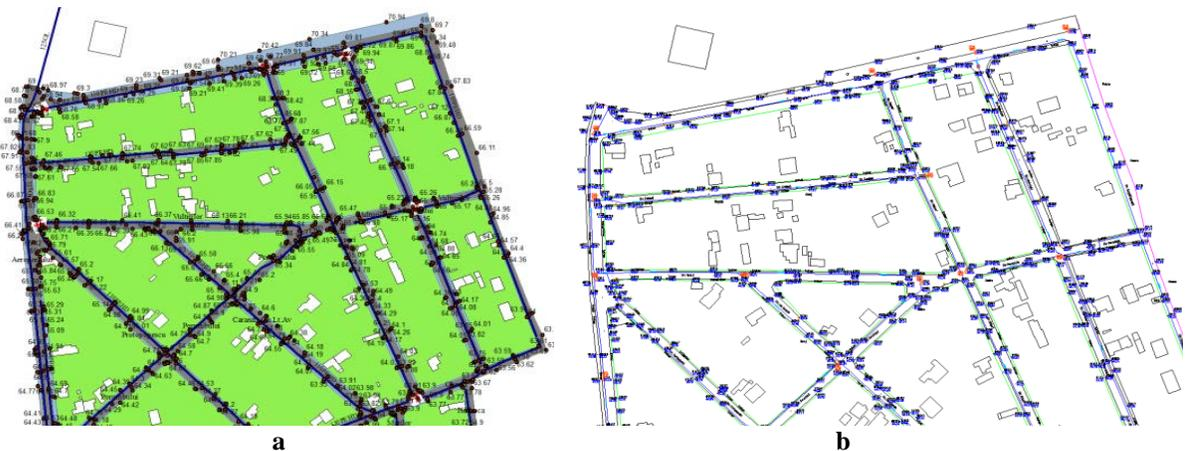
**Figure 1. Viewing the GIS model in different programs: a – ArcMap; b – Autocad Map 3D**
