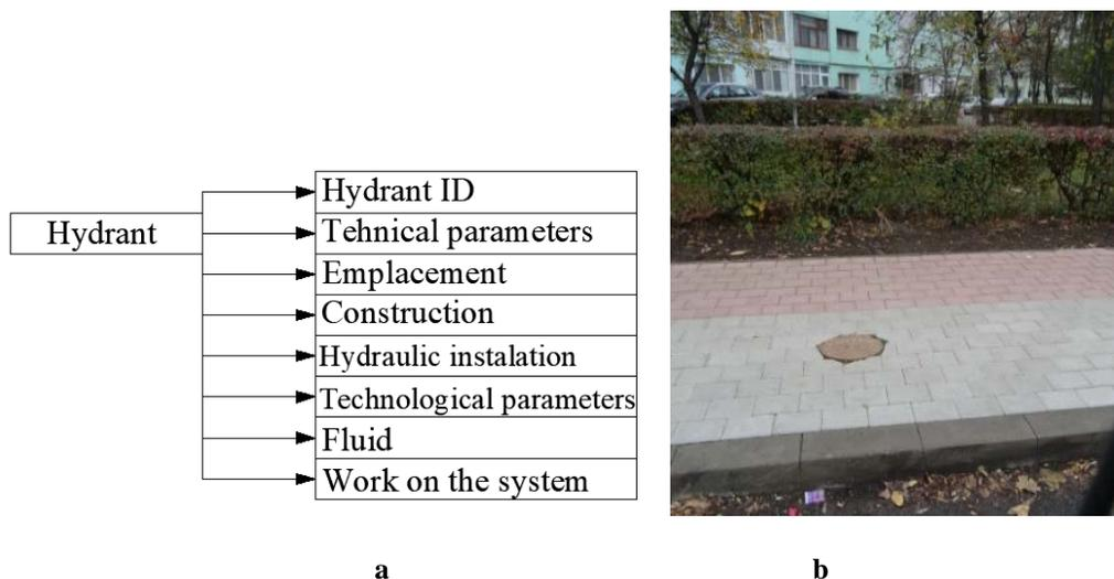
**Figure 3. Characteristic data for the street hydrant network: a - the set of layers for characterization hydrant in the GIS model; b - street hydrant mounted on the rearranged (sidewalk) traffic area**
