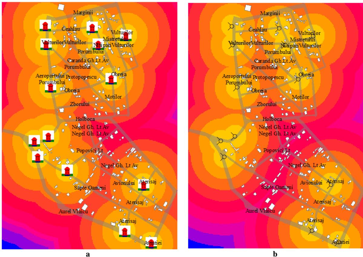
Figure 6. Fire hydrant coverage range: a - Scenario 1; b - Scenario 2
