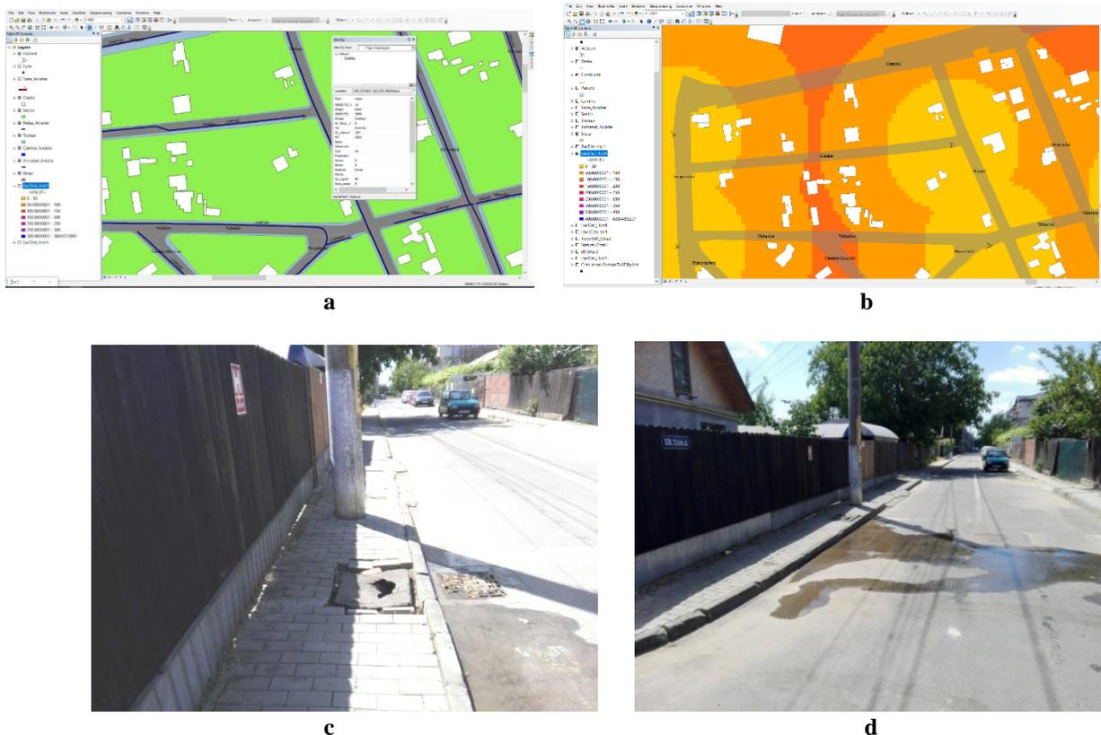
**Figure 4. Hydrant identification of H6: a - Viewing textual data in ArcMap; b - Visualization of fire area coverage; c - detail on the state of the hydrant; d - general view of Ceahlau str., Iasi**
