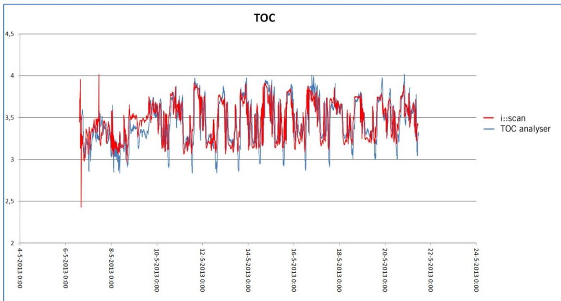
Figure 5. Measurement results of the i::scan absolutely keep up with those of traditional TOC analysers that cost 5 times more and requires high maintenance
