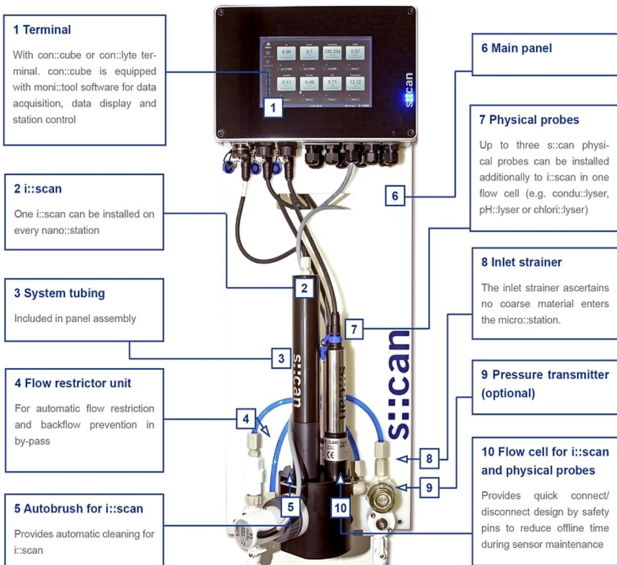
Figure 2. The nano::station combines the i::scan with additional sensors for pH, chlorine and conductivity
