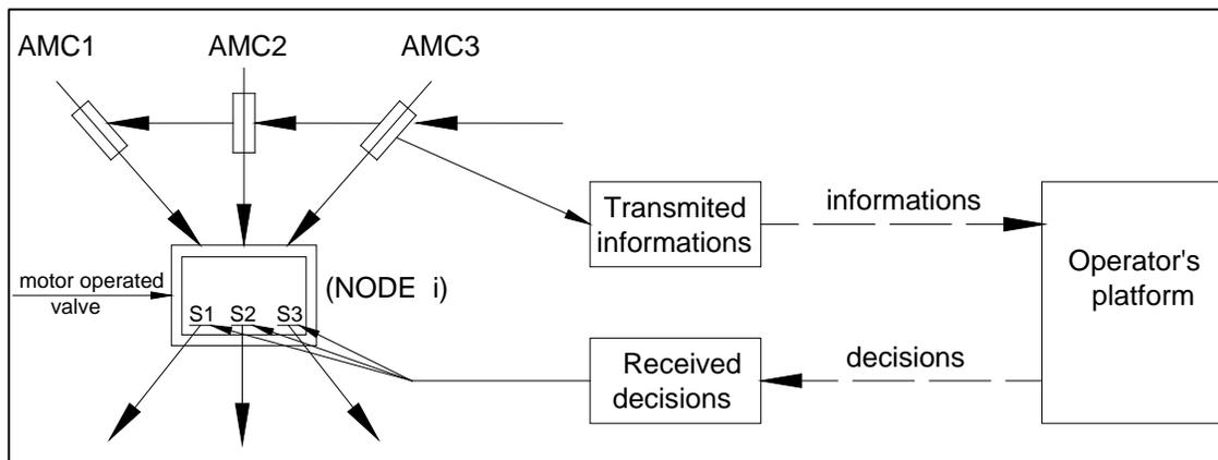
Figure 3. Equipment of a NOD with input flow meters and adjustment devices
