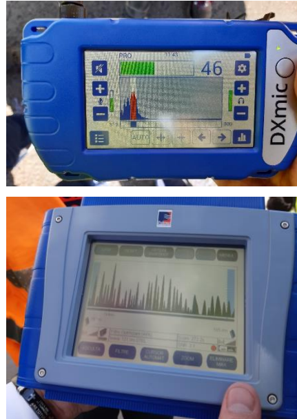
Development of active leakage detection as a daily activity to find invisible bursts
