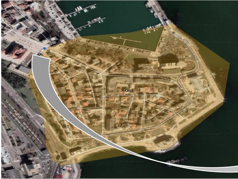
Flow metering at the entrance of the DMA and data communication (datalogger) to a central database
